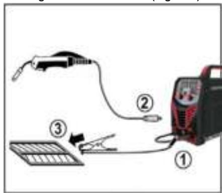
**Welding with an electrode (Figure 3)**
