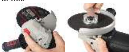
Lock the grinding spindle with the spindle lock button before clamping and releasing the abrasive tools.
